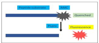
The assay is fast and convenient, and requires just two steps. In the first step, the PLpro enzyme is preincubated with the compound for 30 minutes. The reaction is initiated by adding substrate solution at the second step. Fluorescent intensity is measured with a fluorescent plate reader at the excitation wavelengths of 340-360 nm and emission wavelengths of 460-480 nm.
